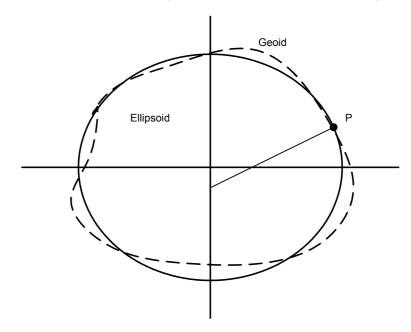
Fig. 1 Measuring the position of point P in terms of a reference ellipsoid.
