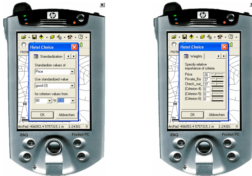
Figure 2: ArcPad™ desktop emulation showing the standardization of criteria (a) and the definition of relative importance weights (b) by the user.
