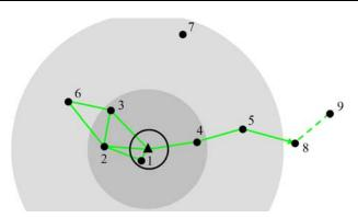
**Fig. 1.** A client agent (triangle) requesting help via short-range radio and the emerging communication network
