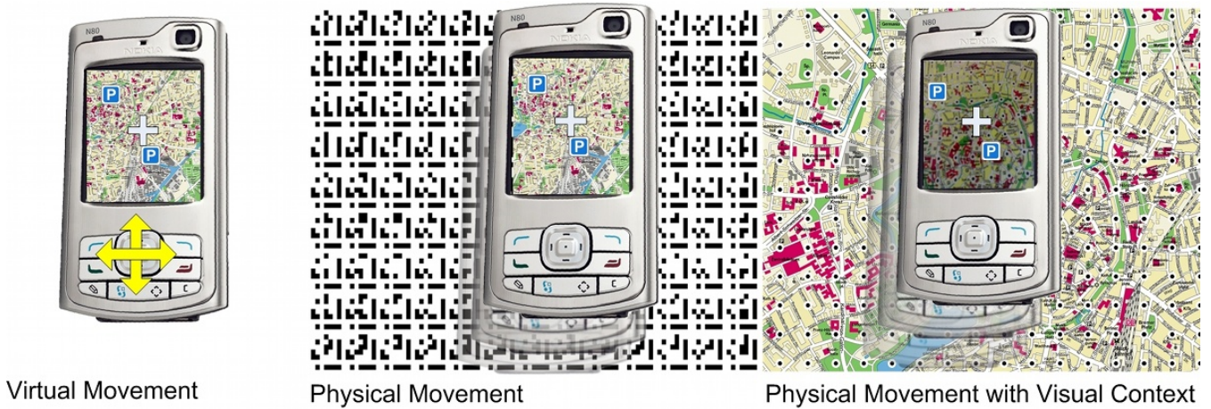
Figure 2: The investigated map navigation methods: in the static peephole interface the virtual map moves while the physical device is static (left); in the dynamic peephole interface (middle) and the magic lens interface (right) the physical device moves and the virtual map is static with respect to the background.
