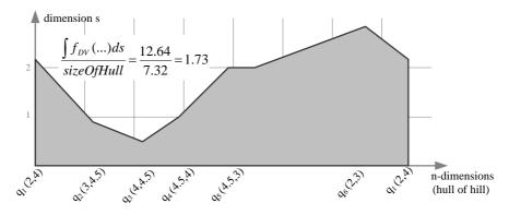
Fig. 7. Transformation of the pointwise Euclidian distance values into one distance value.
